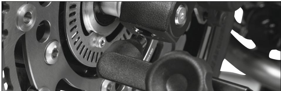
The paddock stand supports for open fork tubes must be adjusted to the width of the front fork. To do so, a second person must hold the handlebars straight. Position the supports under the motorcycle's fork tubes from the front. Adjust the supports so that they fit fully under the two fork tubes, and fit the adapters into the opening/hole in the fork tubes. Make sure the adapters are a good fit in the opening and do not have too much play. Secure the supports with the star grips.
