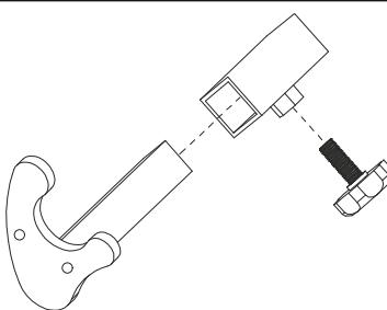
Then connect the suitable adapter for the respective motorcycle to the corresponding supports inside and gently tighten them with the star grip. The paddock stand is suitable for a support width of approximately 270 to 370 mm.
