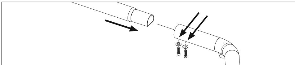
The paddock stand first has to be assembled before it can be used. To do so, the two jacking arms are inserted into the connection tube and screwed in place from below on each side with two hexagon socket screws (wrench size 4) and washers.
