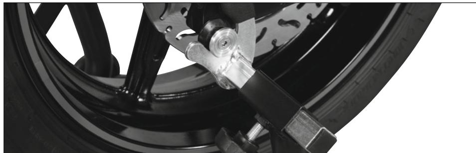
First check that the swing arm is fitted with bobbins that are suitable for the Rothewald Paddock Stand and that they are securely screwed in. If your motorcycle does not have bobbins, you will need to purchase a set and install them in the internal threads on the swing arm.
