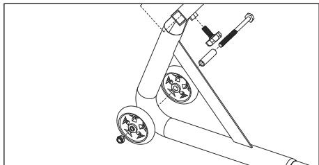
Then connect the spacer sleeves to the wheels. Position the wheels on the left and right, next to the axle mount. Then insert the bolt from the outside, through the wheels and the axle mount and fasten it with the nut (wrench sizes 13 and 14 mm are required). Then connect the cap to the nut. Repeat the indicated steps on the other side.
