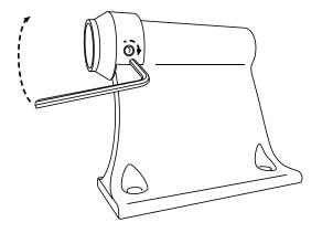
20x100mm and 20x110mm plugs fit *over* the HUSKE base rather than in. Slide the plugs over the top tube, matching the slots to the sides of the base. Once fully seated, tighten the set screw on each plug with a 2mm Allen wrench.
